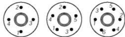
Lug nuts (or bolts) are tightened as shown
